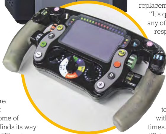
3D printing steering wheels allows the complicated layout of buttons to be optimised for drivers
